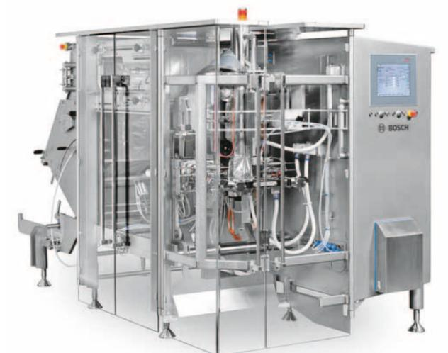
Mydibel's rigorous attention to delivering first-class products has helped the business grow exponentially. With the SVC 4020 the company is well positioned to keep up with increased production demands. "The SVC 4020 is 20 to 25 percent faster than the previous generation of vertical baggers and technologically more advanced," adds Mylle. "It reduces product waste and downtime."
